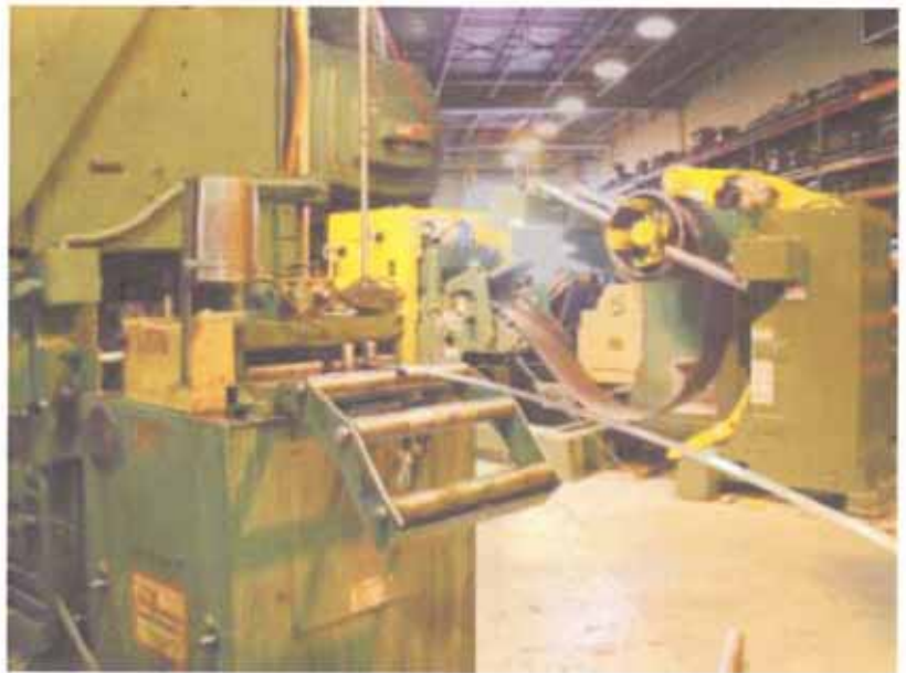
Two press COE feed lines at Manor Tool and Manufacturing: background is the newly installed SpaceMaster Compact Coil Line, foreground is an older servo roll feed that's been in operation for more than a decade.
