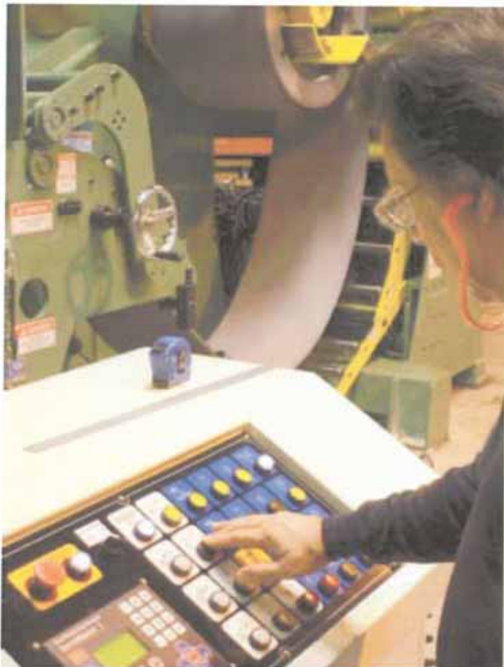
The Coe SpaceMaster Compact Coil Line (Series 3) used at Manor Tool and Manufacturing...close up of the ServoMaster Control unit of the machine.
