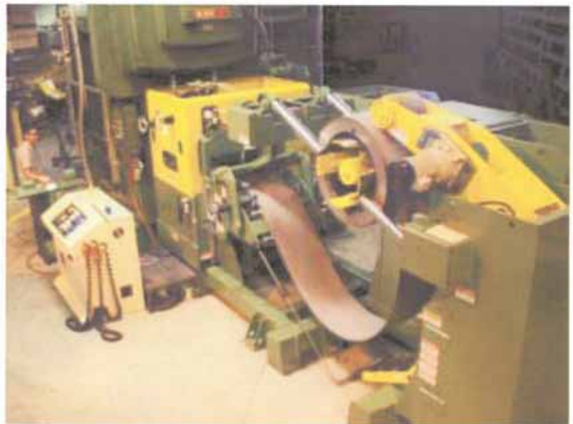
The Coe SpaceMaster Compact Coil Line (Series 3) used at Manor Tool and Manufacturing.
